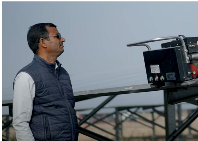
Nirmal Das Swami, owner of Sawarda Solar Farm, observes a robotic solar panel cleaner. Badwali Dhani, Rajasthan, India. (Photo courtesy of GEAPP)
